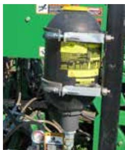
For farming over terraces, especially when using only a single rank of openers, Exapta offers an optional 2.5-gallon accumulator for UniForce on air drills. For 2 box drills together on a hitch in terraces, we have 1-gallon accumulators (one for each drill). When hitting terraces square-on (angle isn't a problem), even the highest-capacity tractors can't supply enough oil flow to keep the pressure perfectly constant, but our accumulator helps minimize fluctuations.
