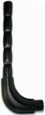
Smallaire riser pipes have an enlarged elbow to properly disperse product going up to the distribution head (ordinary mandrel bends cause ricochet and overload one side of the head). Dimples also help this. Tremendous durability. Smallaire are the wizards of air flow. Reap the rewards of a uniform amount of product going to each opener.
