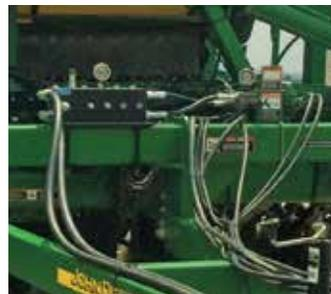
UniForce uses single-action cylinders along with the OEM rockshaft, which is still used to raise and lower the openers. Both can run on a single tractor remote, or they can be kept entirely separate.
