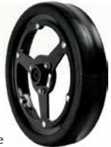
MudSmith gauge tires are 40% thicker, for 20 – 80% longer life. Gauge tires are semi-pneumatic, and pliable compared to some of the rock-hard ones on the market (more sidewall compaction). Super-rugged rim and hub. Available in 4.5" and 3" widths. 2.5" are available, but are not semi-pneumatic, and only for use with twin-row planters.
