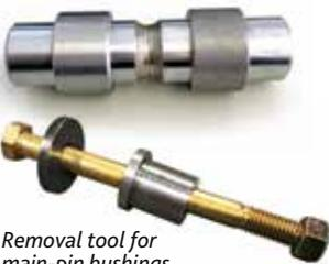
Removal tool for main-pin bushings
