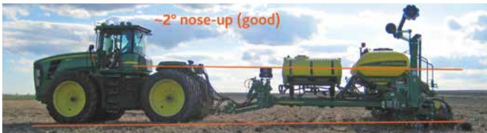
**Step 1, Cut:** Avoid disturbing the path of the opener. If your planter has coulters, run them really shallow—like 6" above the soil! ☺ Fertilizer openers should run approx. 4" to the side, and no deeper than the seed openers (preferably shallower).
