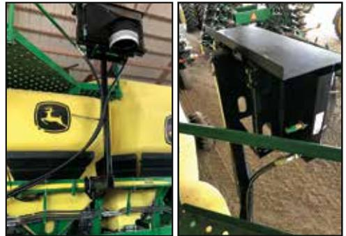
Exapta's Smallaire Heat Exchanger is designed by air movement specialists and has a proven track-record. When cleanout is needed, there's easy access with the hinged cover. The Smallaire unit has a huge radiator (24" x 28", and extra thick), and a plenum to utilize the full extent of the radiator area, so you get maximum cooling of oil and maximum warming of air in the system — great for tough conditions. (Ducting not yet installed in photos.)
