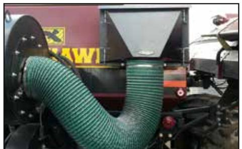
*Smallaire Heat Exchanger mounted on a SeedHawk using flexible ductwork. Usually, the heat exchanger is mounted in a convenient spot on frame tubing using U-bolts.*
