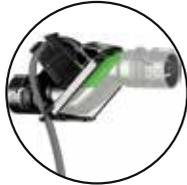
**2.** The seed impacts a stainless steel membrane, creating a small pulse of sound that travels out through an auditory tube.
