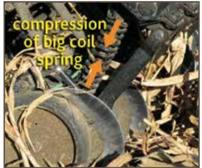
*Inadequate down-pressure causes shallow furrows and more misplaced seeds. The only meaningful indicator of down-pressure is compression of the big coil spring.*
