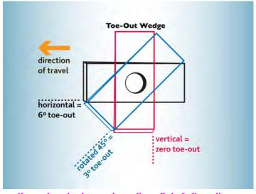
the toe-out to 3 degrees – a good starting place for mellower soils, such as in the northern Corn Belt & Canadian prairies. Install closing wheel using original spacers & bolt. Hold wedge in place while tightening bolt. The wedge won't turn after bolt is tightened. [Note on JD 1700-series: it may be desirable to place a flat washer under the locknut on inside of closing bracket, to help distribute the load since bolt is now at an angle and the cast material is slightly brittle.]
