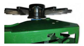
Remove closing wheel & spacers. Place wedge with wide end towards front of planter for the full 6° of toe-out (a suggested starting place for setup for soddy conditions or tough clay soils that resist closing, such as southern USA), or rotate the wedge by 45 degrees (see diagram) to reduce
