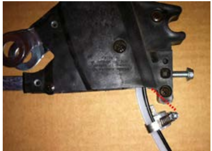
For Wave tails, grind off bracket at red dashed line.
