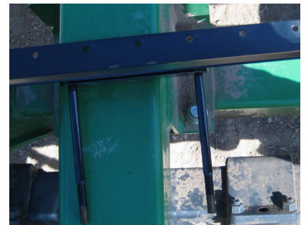
Photo E. RH wing, front, outer end (on 40-ft drill). Tray attached via \frac{1}{2} x \frac{1}{2} " buttonhead bolts threaded into U-bracket. Assembly pulled up off the frame tube for viewing. The center section's trays attach the same way.
