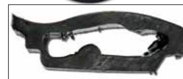
Cross-section of Exapta's PolyFlex tire: high-wear polyurethane with a hollow core, that can flex.
