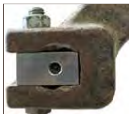
No need to replace worn depth adjustment arms with the new solid axle shaft.
